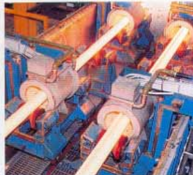
Horizontal conical roller mill in the Pinteg Works of British Steel Stainless.
